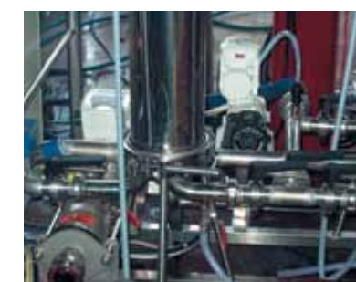
Pump on filtering pallet (wine production).
