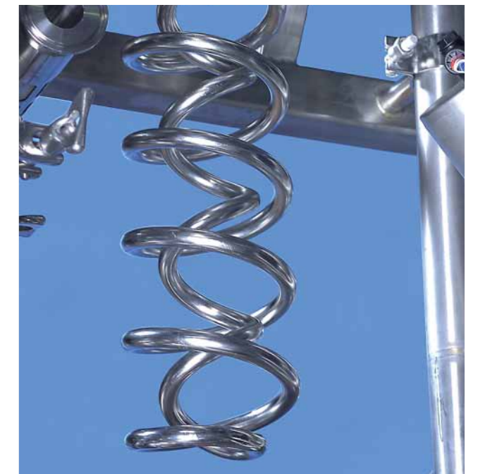
Low shear screw profile preserves product texture
