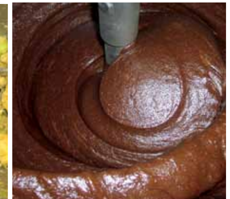
Transfer of highly viscous chocolate for injection in a dessert using the PCM Viscofeeder™.
