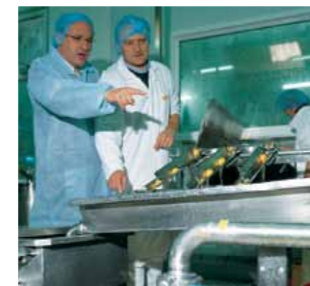
Transfer of egg yolks using a PCM pump in an egg breaking plant.
