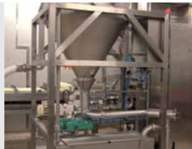
PCM Viscofeeder™ used to dose dough in industrial baking
