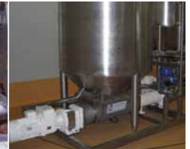
Hopper pump connected to a storage tank
